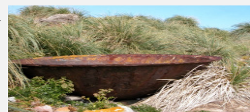
A tri-pot for rendering oil, examples can still be seen today on islands such as Steeple Jason.
