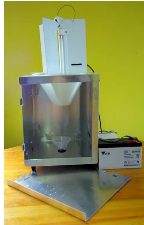
A basic light-trap with one side removed for illustration purposes
