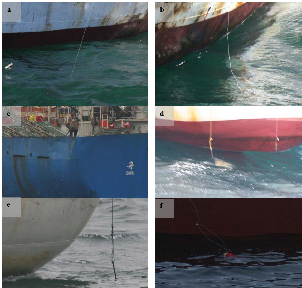
Figure 3: Weighted (a) and non weighted (b) lines used with hooks (c and d) or poles (e) or gloves (f).
