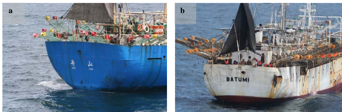
Figure 2: Monofilament (a) and rope (b) used from the stern of the jigging vessels
